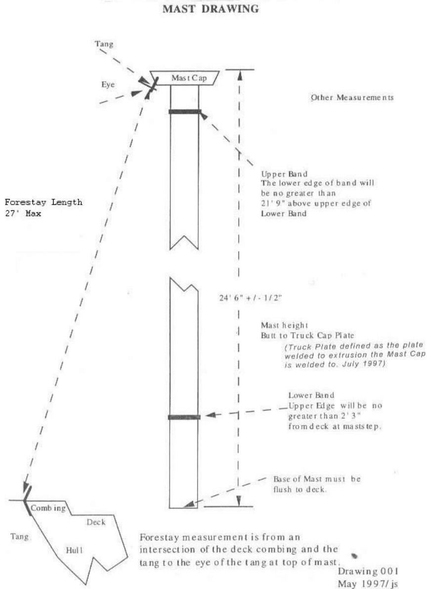
(Truck Plate defined as the plate welded to extrusion the Mast Cap is welded to. July 1997)
